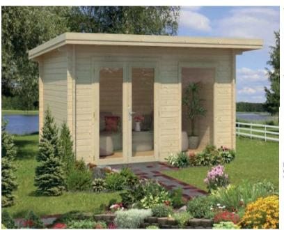
The Idaho 3 is a fantastic looking log cabin, with a similar appearance and style to the Idaho 70mm range of cabins. The building is constructed with 44mm tongue and groove interlocking logs and has a set of double doors and a large single window. The glazing in this building is toughened as standard and is 4mm thick on either side of a 9mm cavity. This building would work great as a home office or summerhouse.
